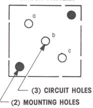
NOTE: THIS ELEMENT CAN BE ROTATED 180° SO POSITION a. b,c BECOMES c,b,a.
